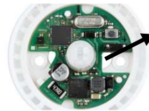
Fig. 6 Remove the KNX terminal. Lead the bus cable through the cable bushing in the base and connect it to the terminal.
