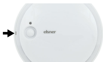
Fig. 3 Open the housing. To do this, carefully lift the cover from the skirting. Start at the recess, e.g. with a flat-head screwdriver.
