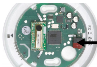
Fig. 6 Connect the KNX bus to the KNX terminal.
