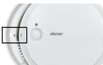
Fig. 7 Close the housing by positioning the cover and snapping it into place. To do this, align the recess on the cover to the marking on the skirting (Fig. 1+2: A).
