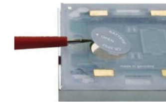
Fig. 6 Carefully pry the battery compartment on the rear of the switch open using a screwdriver. Start on the side with the arrow.
