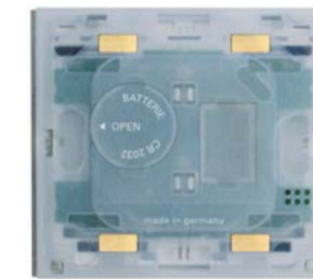
Fig. 8 Then replace the cover of the battery compartment; the arrow must point outward. Press the cover down firmly so that it engages. Place the switch unit into the frame.
