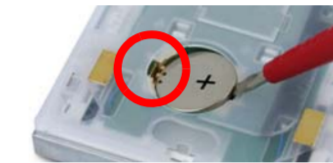
Fig. 7 Pry the flat battery carefully from the bracket. When inserting the new battery, pay attention to the brackets and the polarity (+ must be visible).
