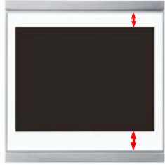
Fig. 5 The display unit can now be put in place. The wider part of the display edge must be at the bottom. The display unit engages on the right and left sides and is also held by magnets.
