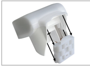
Fig. 16 Push the housing from above into the fastened mount. The bumps on the mount must snap into the rails in the housing.
