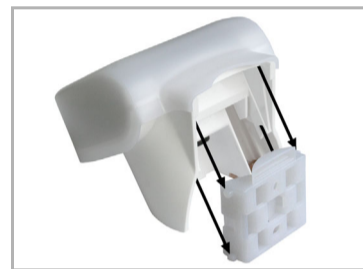
Fig. 12 Push the housing from above into the fastened mount. The bumps on the mount must snap into the rails in the housing.
