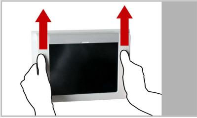
Slide the upper part of the WS1000 Color housing (frame with display) slightly upwards and lift it off.
