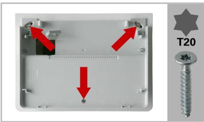
The lower part of the housing, including the wall mounting plate, is fixed to the concealed box by 3 screws: Loosen the screws and remove the lower part.
