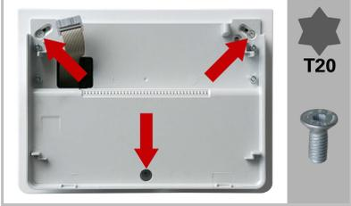
Also pull the display cable through the recess in the WS1000 Color wall mounting plate and screw the lower part onto the adapter plate (3 M4 countersunk Allen screws are provided with the adapter plate).
