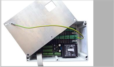
Connect the adapter plate earth with the WS1000 Color circuit board. The protective conductor can be connected to the PE terminal for the mains connection or to a vacant drive group of the WS1000. Alternatively, a protective conductor terminal on the building can be used for earthing.
