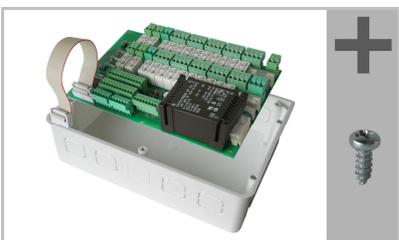
Remove the circuit board from the WS1000 Color. Place it in the concealed box of the old WS1000.
