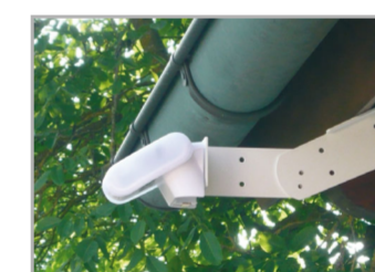
Fig. 8 Example use of the hinge arm mounting: With the hinge arm mounting, the weather station projects from beneath the roof overhang. Sun, wind and precipitation can act upon the sensors without hindrance.
